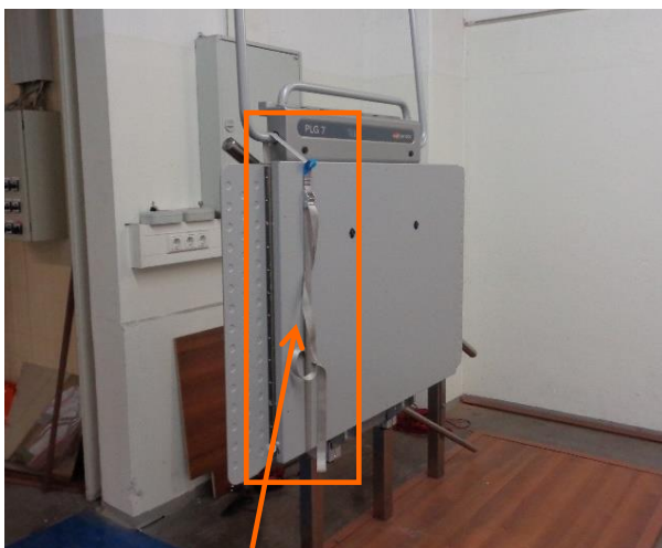
Pay particular attention when tightening the belt not to scratch the lift surface!
