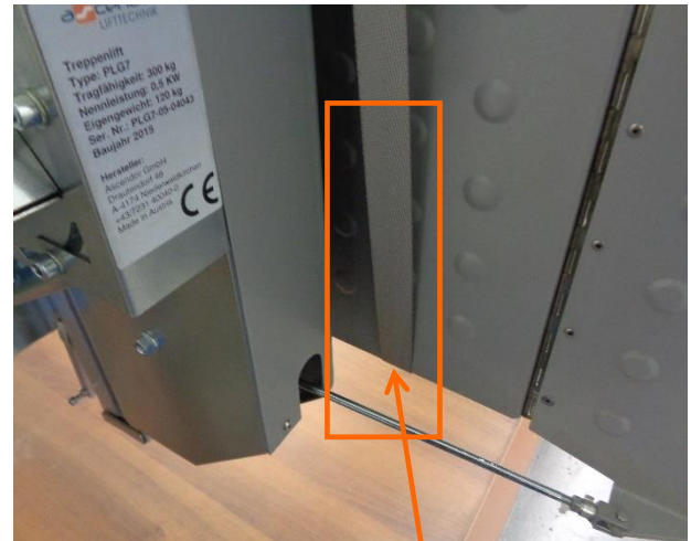
Insert the tension belt between platform and threaded rod at the bottom of the lift.
