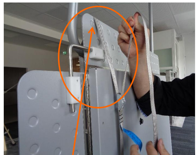
Where a front mounted access ramp is fitted, pass the belt over the top edge of the ramp.
